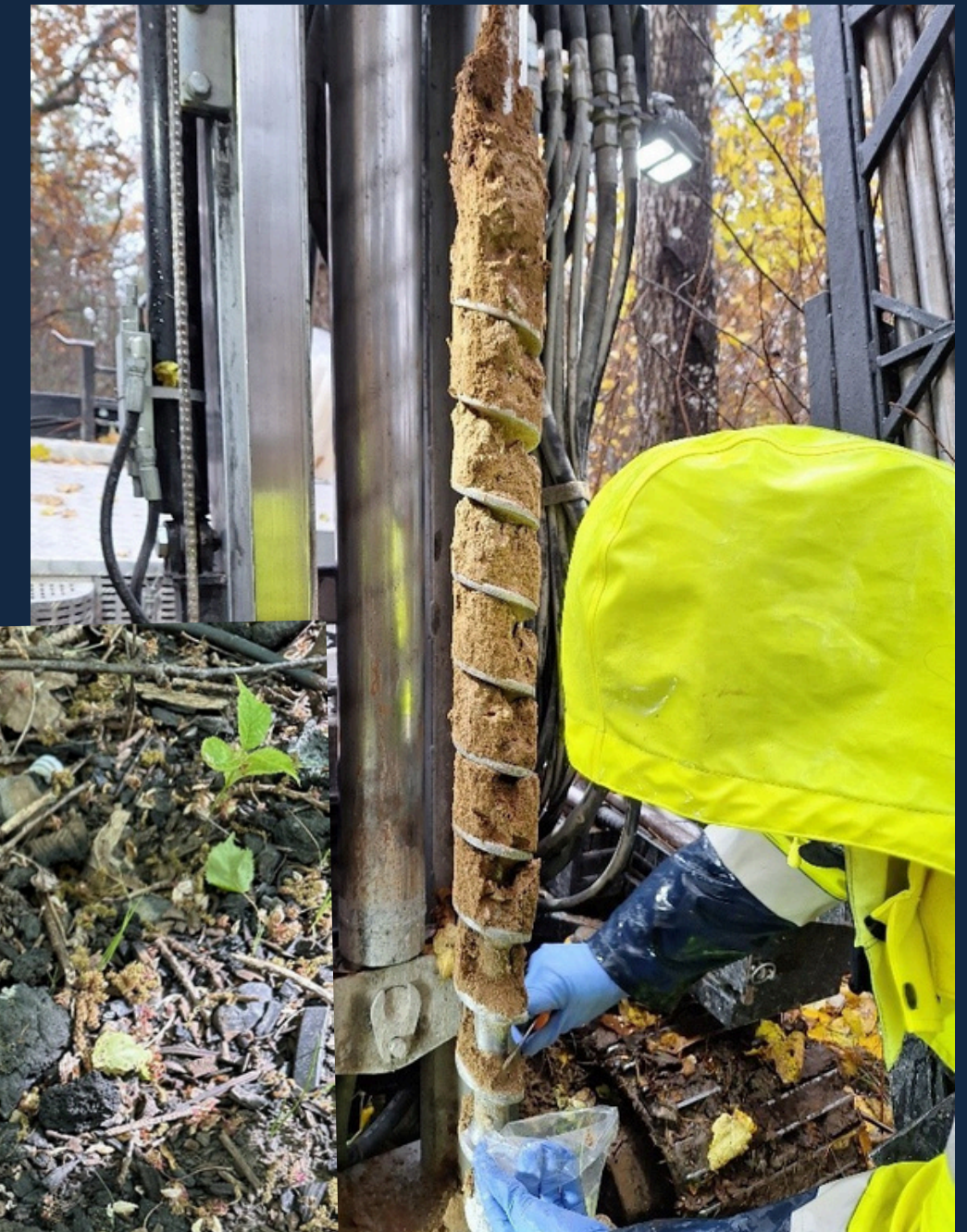
Pictures 8 and 9. Contaminated soil and environmental soil sampling with Mittas drilling rig.
